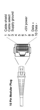
Use of a cable with improper pin assignments may lead to damage to the unit. Use of any cables not provided by the manufacturer may result in damage not Pin assignments are not compatible with Honeywell legacy products. covered by your warranty. Note:
